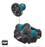
ADD THIN LAYER OF GREASE TO INTERNAL GEARS (NOT SPUR GEAR).
