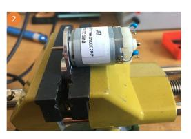
Attach Aluminum Motor Holder to DC Motor according to manual (p. 26 Step 4), DO NOT INSTALL MOTOR WARNING: use max M2x5 screws to attach motor
