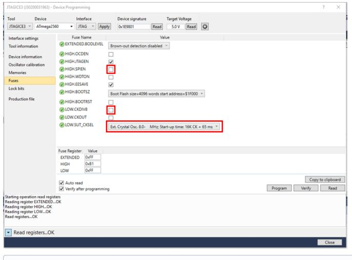
f) If vehicle is behaving irregularly i.e. servo steering is acting erratic, LEDs timing appears off, this is most likely due to an issue with the clock.
