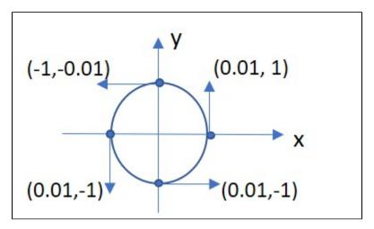
Now implement your points and speed values using the predefined vetors  $trajectory_px$  and  $trajectory_py$  for your points of the trajectory and  $trajectory_vx$  and  $trajectory_vx$  and  $trajectory_vx$  for the speed at each point. The speed is given in m/s. Set the center of the circle to the center of the map at x = 2, 25m and v = 2m.
