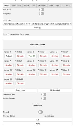
The setup view allows to launch all components required to perform a simulation from within the LCC's GUI. It can also be used for real vehicles, and to deploy your selected program or script remotely on the NUCs (HLCs).
