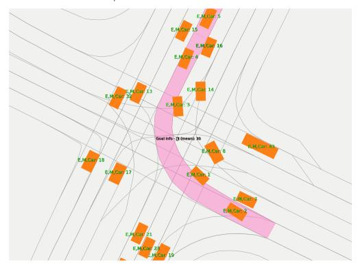
You can see an example of a simulation in the Gif shown above. Vehicle 4 was chosen to be represented by a real vehicle, so upon starting the scenario, the vehicle is replaced by a trajectory that is sent within the network. You can find out more about this in Commonroad Tab.
