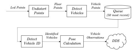
The **UndistortPoints** function transforms the image/pixel coordinates to metric coordinates on the driving surface (floor). The calculation is based on a calibration image. See https://github.com/embedded-software-laboratory/cpm-lab/tree/master/matlab\_scripts/camera\_calibration
