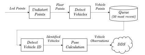
The **UndistortPoints** function transforms the image/pixel coordinates to metric coordinates on the driving surface (floor). The calculation is based on a calibration image. See https://github.com/embedded-software-laboratory/cpm-lab/tree/master/matlab\_scripts/camera\_calibration
