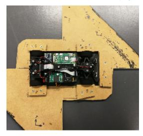
While the IPS is running, the vehicle is placed in various poses on the floor, following a particular calibration sequence. The calibration features (back\_x, back\_y, direction\_x, direction\_y) are recorded from the running IPS. A linear calibration is then fitted using least squares.
