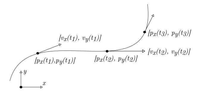
The time between trajectory points t(i+1) - t(i) is not fixed, but should be between 100 ms and 400 ms. Due to network latency and the controller structure, the trajectory points need to be created and sent ahead of time. The exact required lead time is TBD, but 1000 ms should be enough.
