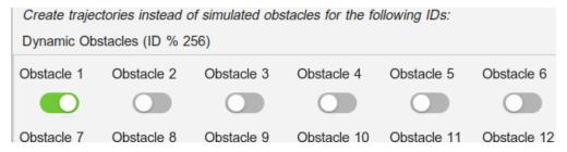
In the image above, the path of obstacle 1 is communicated in form of trajectory messages for vehicle 1 - which can also be received and followed by a real vehicle - while the other obstacles are simulated without controlling real vehicles.
