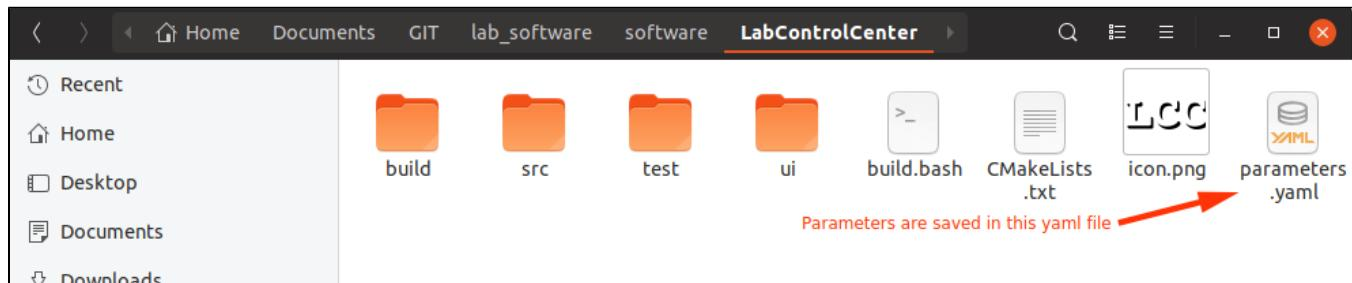
The parameters are stored in the YAML format in the file `parameters.yaml` in the directory of the LCC. Some parameters are distributed on program startup, these must be either edited in the LCC before restarting it, or they can be edited manually by changing the content of the YAML file:
