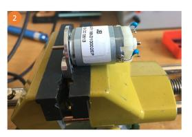
Attach Aluminum Motor Holder to DC Motor according to manual (p. 26 Step 4), DO NOT INSTALL MOTOR WARNING: use max M2x5 screws to attach motor
