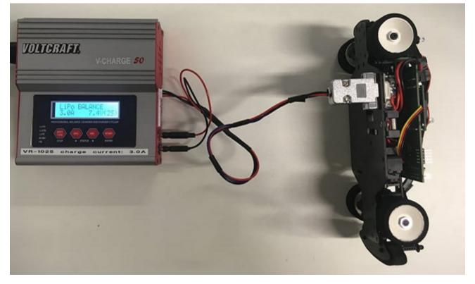
Turning off the vehicle is important so that charge termination is successful. LiPo chargers work by charging in two modes, first constant current (CC) then constant voltage (CV). During CV, the current is monitored until it drops under a certain threshold at which point the charger terminates the charging process. If the vehicle is left on, this threshold current may not be reached and the charger will charge indefinitely.
